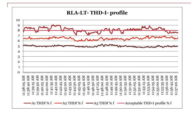
The percentage of average current THD is in the range of 5.0 % to 9.0%. The current harmonics in the system are more than the recommended limits as per IEEE Standards.
